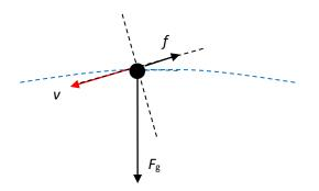
The much bigger gravitational force has a component *along* the velocity. This increases the satellite's speed while the frictional force decreases it. Overall, the speed increases.
